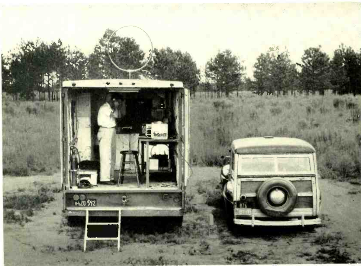
Fig. 8—Thunder hunting equipment on location near Madison, Florida. Loop antenna picks up static which is fed into wide band recorder.
