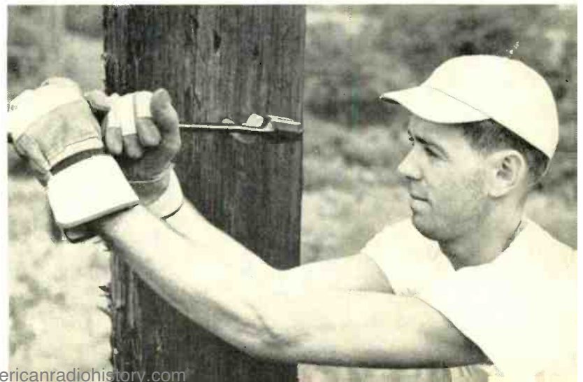
Fig. 3 (left)—Tapered faces of "B" lineman's wrench set wrench shank at an angle to the work so that the shank and the workman's hand clear obstructions as the wrench is turned. Fig. 4 (right)—With the end of the steel pole step in the elliptical hole in the shank, the wrench becomes a lever either for turning the step into proper position or for unscrewing it from the pole.
